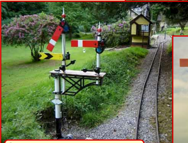
GWR lower quadrant right hand bracket, 2 doll with 2 4ft home arms, fixed distant signal arm and rule 55 diamond
