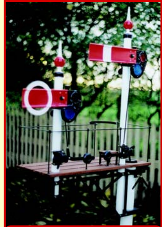
GWR lower quadrant left hand bracket, 2 doll with a 3ft ringed arm and a 4ft arm plus handrails
