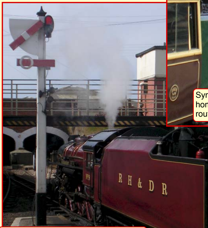
Single post home (or starter) with back-shade, showing proceed aspect and ringed shunt arm.
