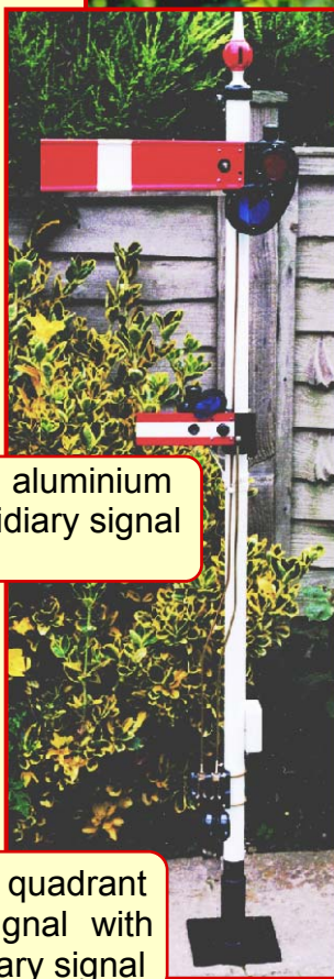
Lower quadrant subsidiary arm mounted on a round post set at clear (proceed)
