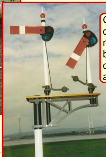
GWR lower quadrant left hand bracket, 2 doll with a 3ft ringed arm and a 4ft arm plus handrails
